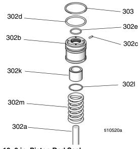
FIG. 18: 3 in. Piston Rod Seal
